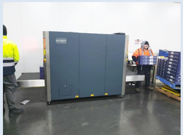
Piece level x-ray examination that the products have to go through in Australia, before they are loaded into the units (in this case, it's an AKE and an AMP).
